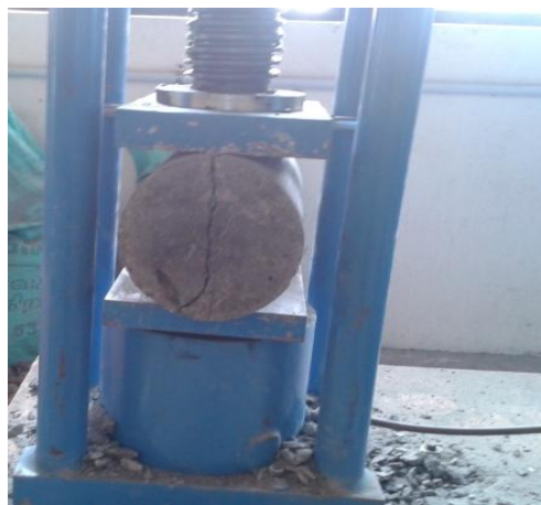
Figure 5: Split tensile Strength Test Setup
