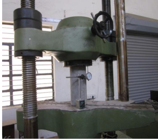
Figure 8.1: Testing of Cylindrical Specimen
