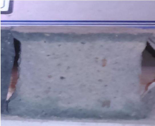
Figure 7.4: Four hours Sulphur Cure
