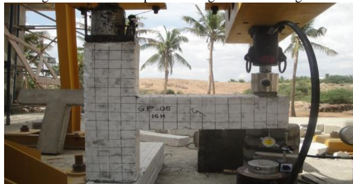
Figure 2: Loading arrangement of beam – column joint
