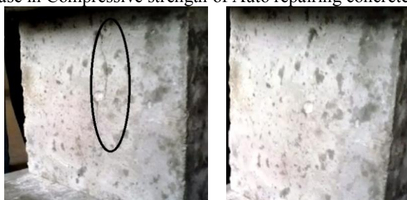
Figure 7: Crack healed concrete specimen with crack (left) &amp; Healed Specimen (right)
