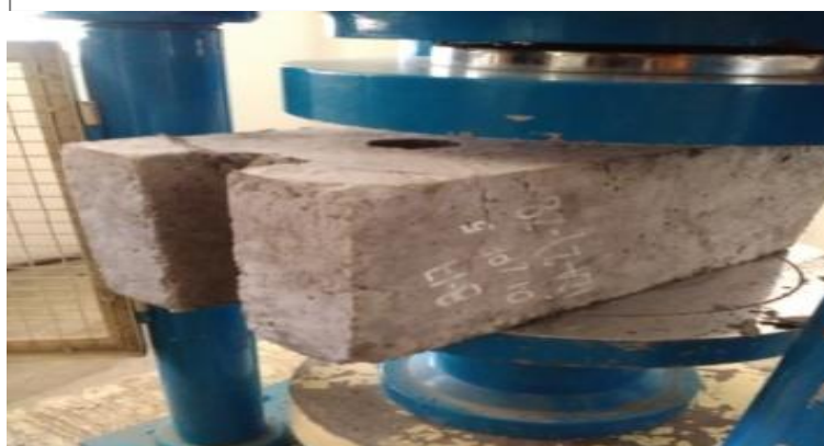
Figure 3: Compression test on hollow block
