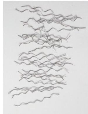
Figure 2 (b): Crimped Steel fibre
