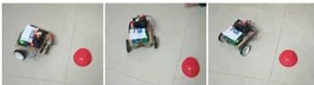
Figure 8: The final robot prototype and its movement by avoiding the obstacle (red color)
